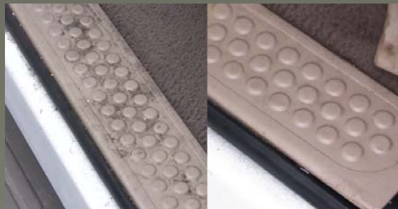
Dirt filled side step
